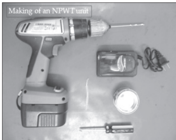
Fig.-1: required materials: One aquarium pump, Screw Driver, Glue, A portion of Infusion set, Drill machine.
